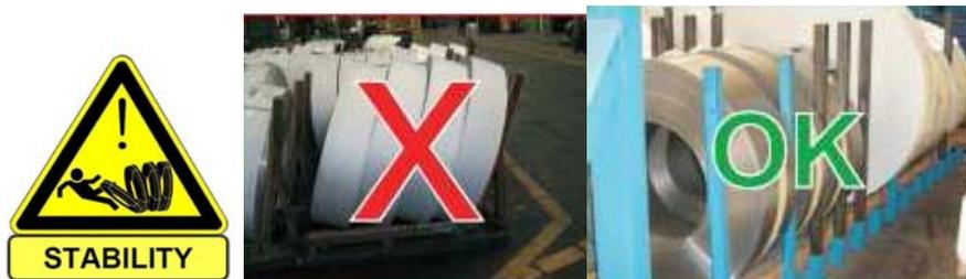
Consequently, adequate equipment must be used to ensure the stability during unpacking operations for coils and/or slitted coils.
