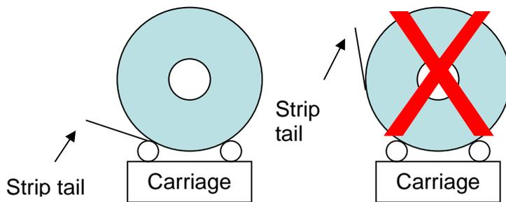
If strap removal takes place on a mandrel on the line, maintain the position of the strip tail by means of the feed carriage or the pressing roll, according to the line equipment and the instructions issued specifically for use of the tool.
