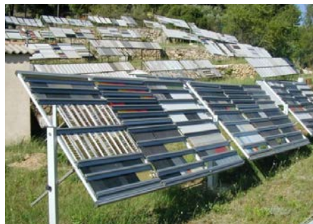
Granite® HDX test panels at the Station d'Essais de Vieillissement Naturel (SEVN) in Sanary-sur-Mer, France. Photograph: © ArcelorMittal Global R&D
