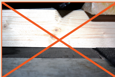
Fig. 2.21 (Bad) The cargo is in contact with the trailer surface (here groove cover)
