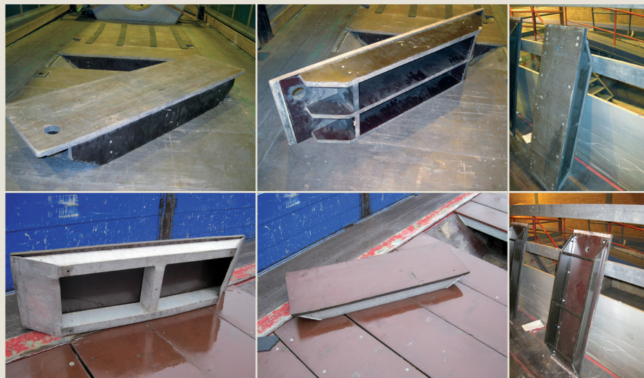
Fig. 2.09-1, 2.09-2, 2.09-3, 2.09-4, 2.09-5, 2.09-6 Examples of recommended types of groove-covers if used as distance holders
