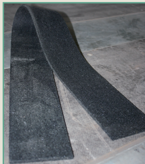
Fig. 2.17 Example of a good anti-slide mat
