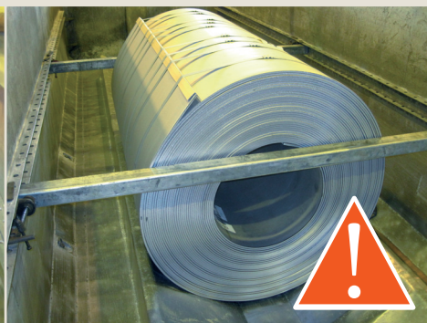
Fig. 1.8 Support structure in front and back of the coil without lashings
