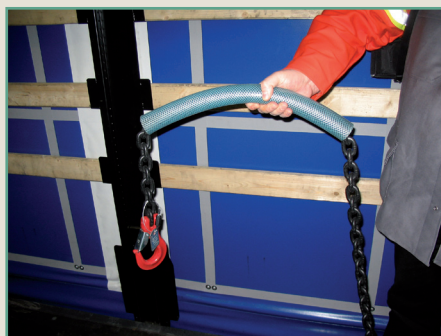
Fig. 2.13 Chain in good condition
