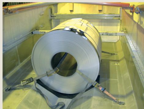
Fig. 1.7 Support structure in front of the coil with lashings;
