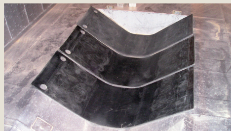
Fig. 2.20 Anti-slide mats for tipper
