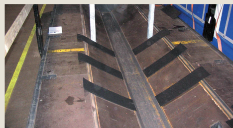
Fig. 2.19 Anti-slide mats in a "normal" groove trailer
