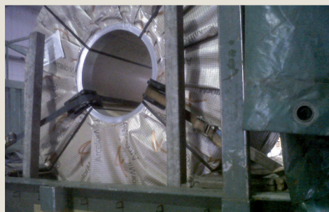
Fig. 1.13 – Case of swap body equipped for receiving the coils with axis transversal to the driving direction; securing is made with two belts and using four corner protections. On both sides, a pair of stanchions must be put.
