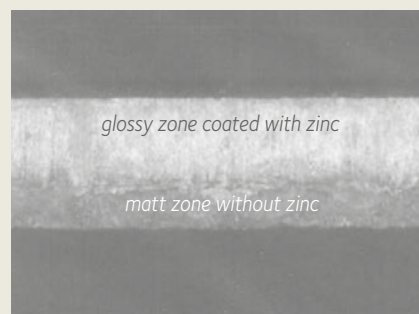
Cut edge (sheared)
