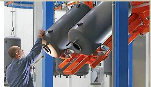
Interior pressure vessel of the Ariston boiler, made with HC300EK
